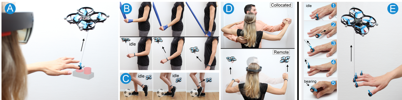
Figure 1: Concept. (A) HapticPuppet drone providing haptic feedback when a user is pressing a virtual button in AR. (B) Demonstrates how the system can be used for exercising. (C) A VR user kicks a ball and feels the impact. (D) A collocated partner dance, and the remote setup using two HapticPuppets. (E) Shows a user's hand augmented with five attachment points.
